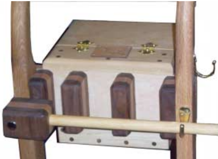
Flip up retaining bar showing "sandwiched" Walnut and Maple blocks
